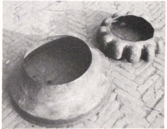
685 Making a pinnacle. The gah with the different hammers to mould the ridge and valleys. Left the bilimugah (hammer) for the middle belt, right the sasmugah and pimugah for the outer edges.
