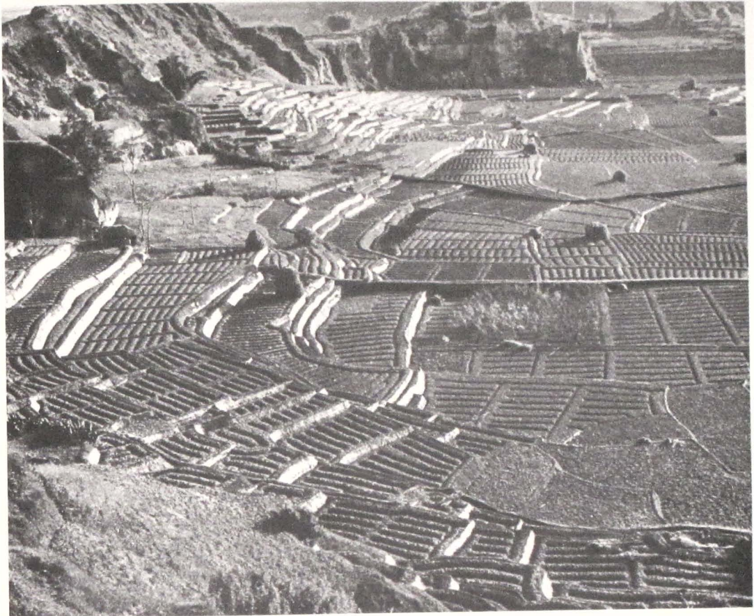
357 The Valley of Kāṭhmāṇḍu provides a variety of clay (cā) and sand (phi) for the production of bricks or to be used as mortar or for whitewashing.
