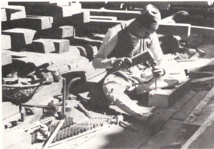
661 Woodcarver (sikaḥmi) with chisel (hā) and mallet (hākhimugah) at work.
