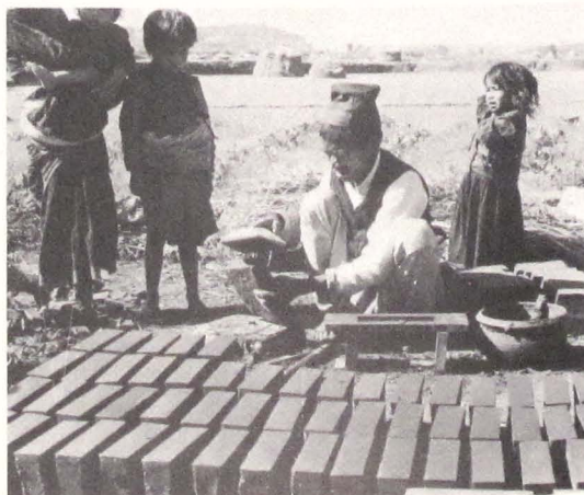
642 Brick maker (āvāh), solidifying the face of conical bricks (dātiapā) with a mallet (bārsā).
