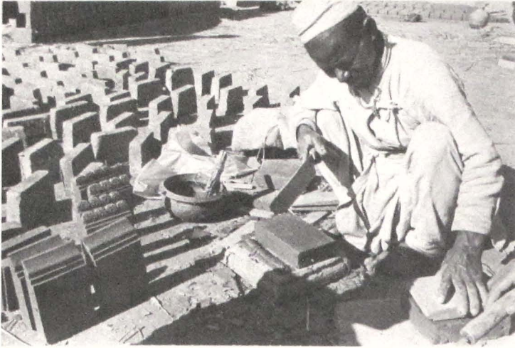
318 The sun-dried (nhaḥ gane – slightly dried) ruffian is cut to size with a knife (syāḥcupi).
