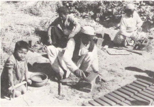
302–307 Finishing of conical bricks (dātiapā).
