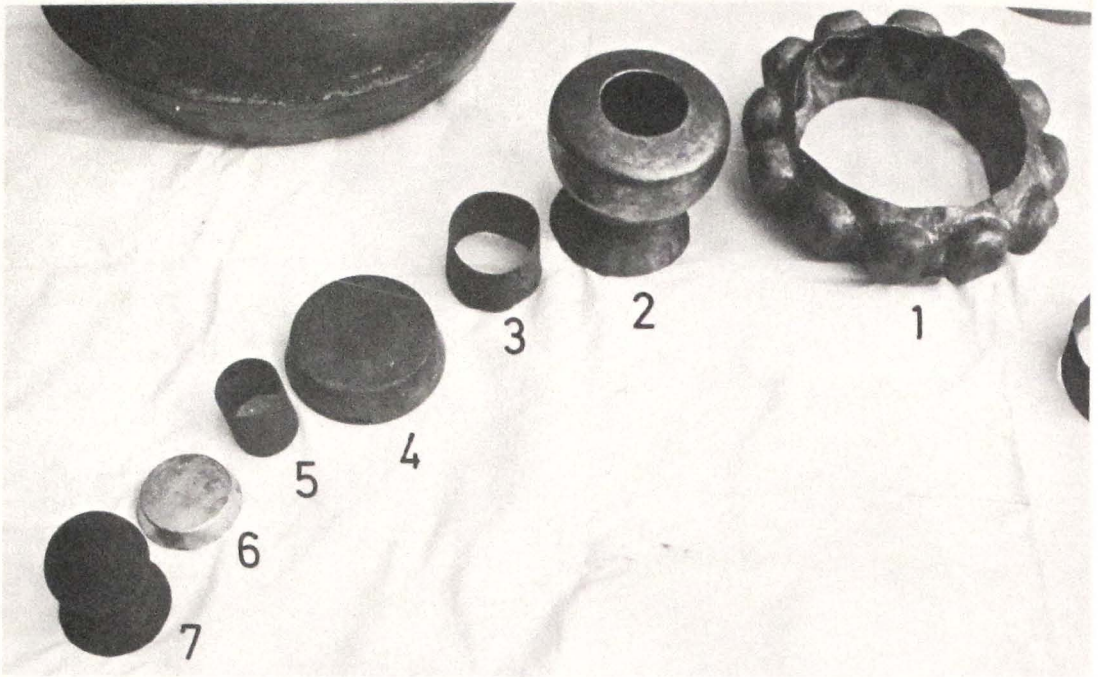
689 Making a pinnacle: the individual parts of the top of the gajū before assembling.
