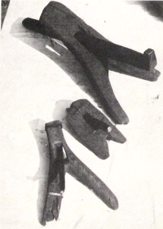
683 Moulding of a base of a pinnacle (gaḥ). The pointed edge of the phecūākhkhalu (anvil) is used to mould the bicklike middle belt. The anvil is inserted into one of the smaller cāgāsī-holders. Bilimugah (hammers) serve as tools.
