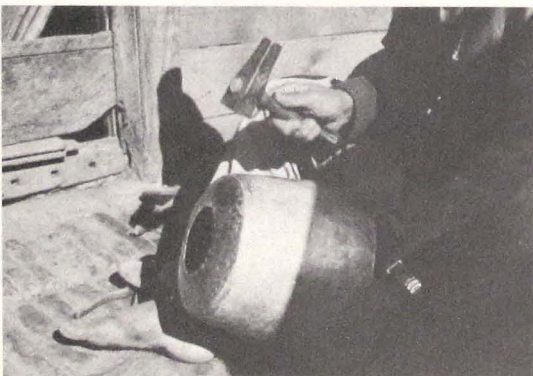
691 Making a pinnacle. The upper part of the ghātākār is placed upon the bvarāḥkhalu and smoothed with a pimugaḥ hammer.
