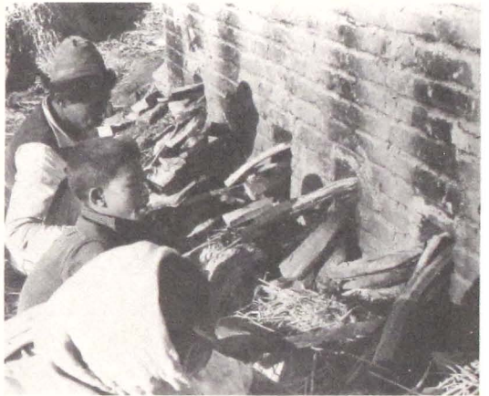
311 Firing the kiln with wood (sī).
