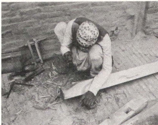
637 Carpenter (sikaḥmi), chopping a beam with an adze (khul).
